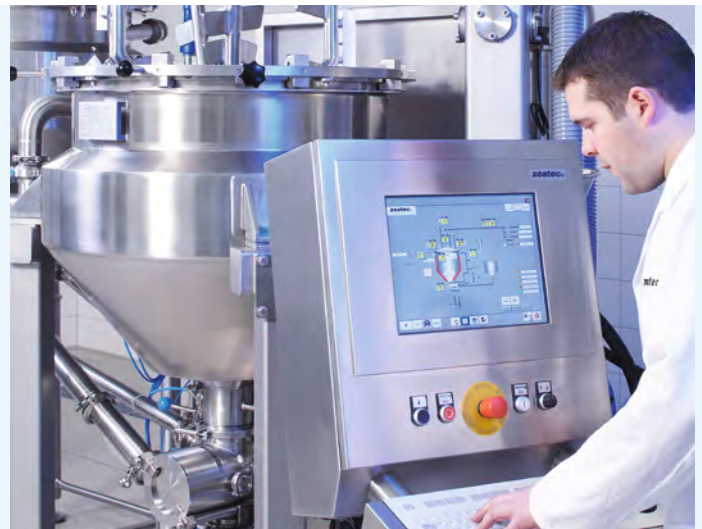
Control terminal with process visualization
