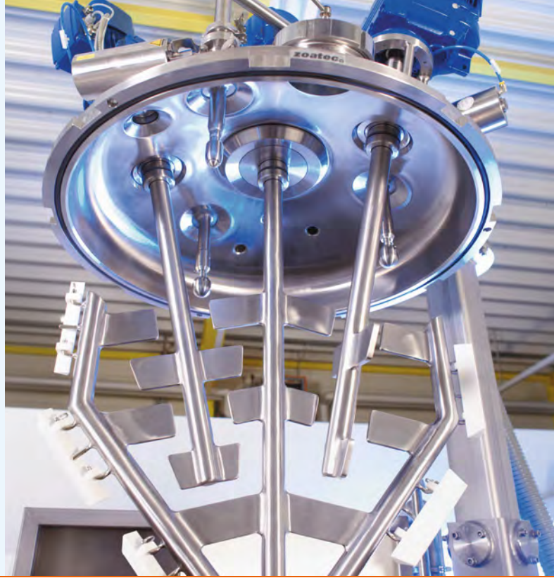
standard agitator 80° with flow breaker
