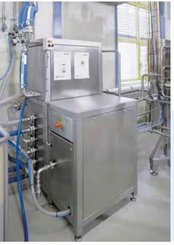
Separate supply unit with pneumatic and vacuum unit and liquid meters
