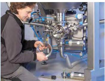
The homogeniser, with pump mode, allows damage-free mixing of chunky goods without using an additional pump
