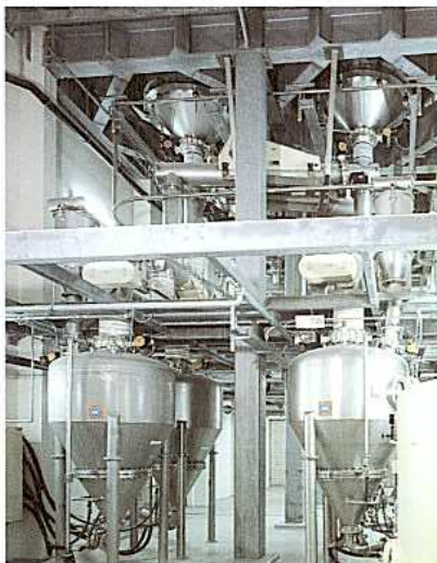
Pressure impulse conveying system for feeding a bag-filling machine and big bag filling
