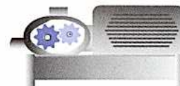
Helical piston compressor For generating positive pressures up to 45 psig. Noise insulation is necessary.
