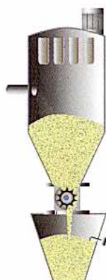
Separator with rotary airlock Used for continuous separation, delivery and simultaneous metering in downstream manufacturing processes.
