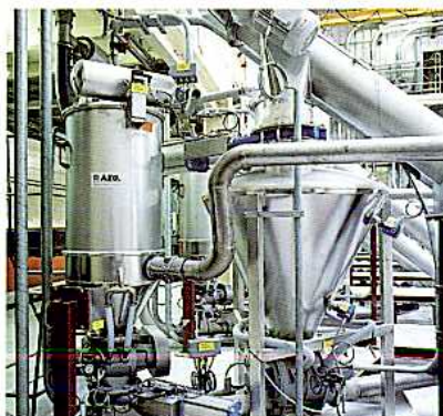
High-pressure airlock for gentle conveying of granular materials
