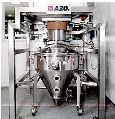
Mobile vacuum hoppers with impulse valve
