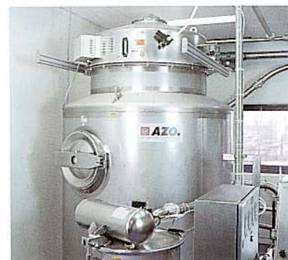
Large filter with service facility
