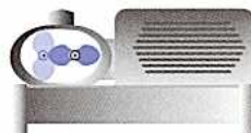
Rotary piston blower For generating positive pressures in conveying systems up to 15 psig. Noise insulation is necessary.
