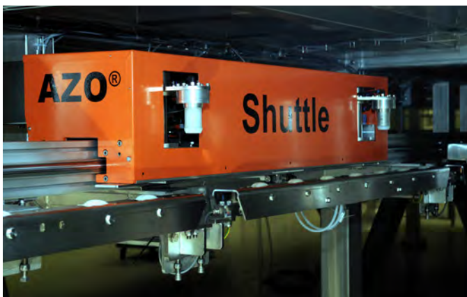
Mobile shuttle units for rapid transport of the collecting containers
