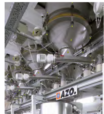
Exact dosing by AZO dosing screws
