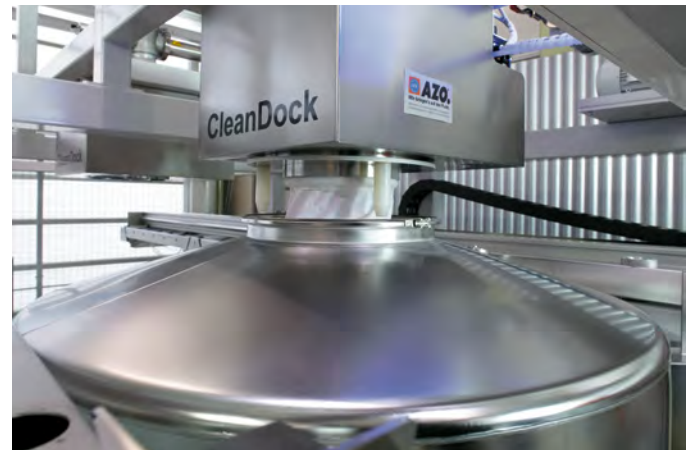
AZO CleanDock® for dust-free docking and undocking of mobile containers
