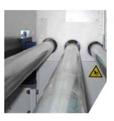
Loading and unloading rollers
