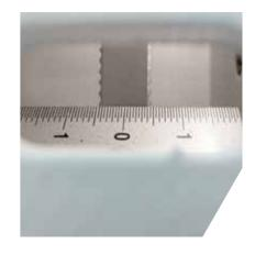
Window for monitoring the knife grinding process
