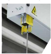
Knife protection unit adjustable by motor
