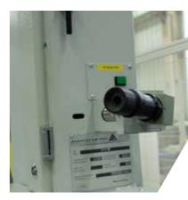
Optical knife grinding control
