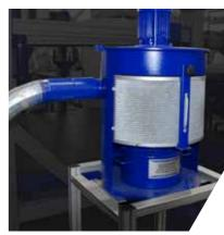
Grinding dust extraction unit
