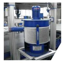
Grinding dust extraction unit
