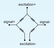
**open-bridge circuit diagram** for uncompensated sensors
