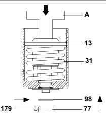
**3.** Fit in the following order the seal (19), the bush (97), the spring (31) and the piston (13) in the cylinder (9).
