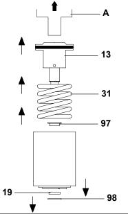
**7.** Having carefully reduced the pressure exerted on the special tool (A) by the spring (31), remove the piston (13) and the spring itself (31). Remove the washer (98), the seal (19) and the bush (97).
