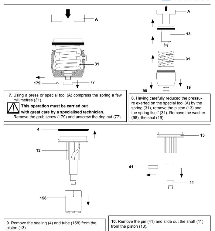
11. Disassembly of valve type ZVF (DN15--100)
