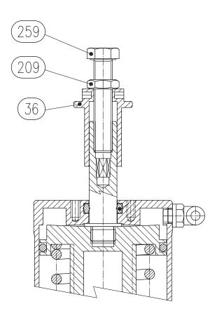
Dismantlement of stroke limiter in outlet
