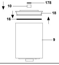
5. Fit in the following order the sealing ring (16), plug (18), bush (10) and sealing ring (178).
