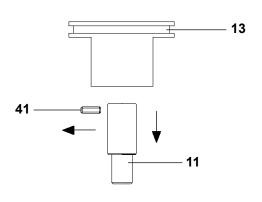
**9.** Remove the pin (41) and slide out the shaft (11) from the piston (13).
