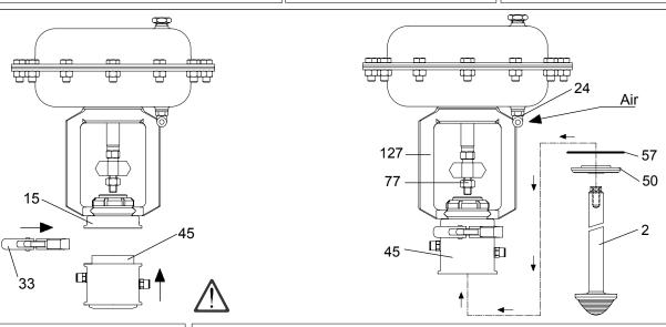
**3. BBYK.** Assemble steam barrier (45) on to head body (15) using the clamp (33).
