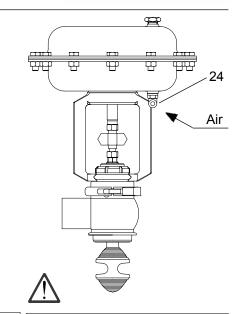
9. Assemble the shutter (30) and the actuator and close with the nut (77)
