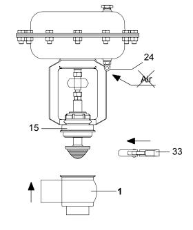
**8. BBYK.** Insert seal rings (156 e 157)\* and guide bushing (120)\* into the cap (50). Fit the cap (50) on the head body (15). Assemble the shutter (2) and the actuator and close with the nut (77). Supply air to the actuator into the air connection (24).
