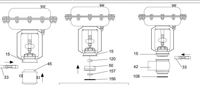
**6. BBYK.** Assemble steam barrier (45) on to head body (15) using the clamp (33).
