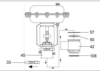
**5. BBYK.** Remove clamp (33), remove upper body (42) and the cap (50) from steam barrier (45). Remove seal ring (57) from steam barrier (45). Remove seal ring (108) from upper body (42).
