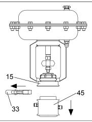
**8. BBYK.** Remove clamp (33) between head body (15) and steam barrier (45). Remove steam barrier (45).
