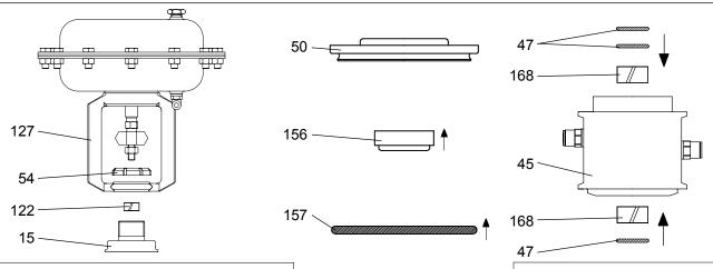
**3.** Fit bushing (122)\* into head body (15). Assemble head body (15) on to the actuator (127) and tighten ring-nut (54).
