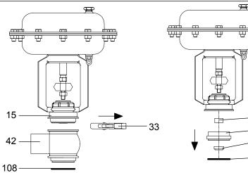
**6.** Remove clamp (33) and upper body (42) from head body (15) remove seal ring (108) from upper body (42).
