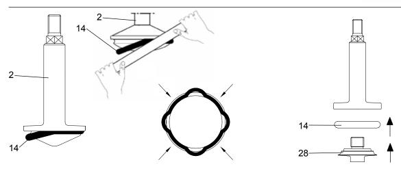
**1.** Pre-heat shutter ring (14)\* to approx. 80°C to make it softer and insert it in shutter slot (2). Insert the ring in a crosswise manner using a plastic cylindrical tool.
