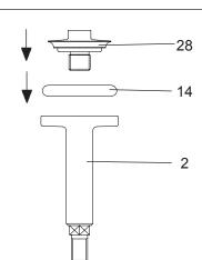
**1.** Pre-heat shutter ring (14\*) to approx. 80°C to make it softer and insert it in shutter slot (2). Insert the ring in a crosswise manner using a plastic cylindrical tool.
