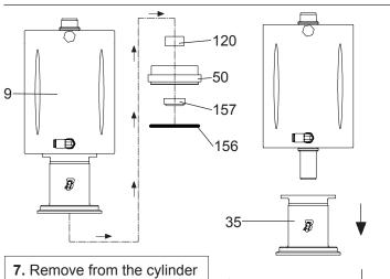
(9) the cap (50). Remove ,from the same, gaskets (156 e 157) and the guide bushing (120).
