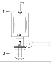
**6.** Screw shutter (2) into cylinder pivot (9). Counterhold the pivot with an allen wrench.
