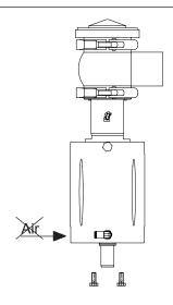
**9.** Insert the sealing ring (191) on the lower body (1). Assemble the lower body (1) to the flange (100) using the clamp (33).
