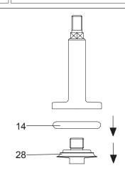
6. P.T.F.E. SHUTTER: Unscrew shutter nut (28) and remove shutter ring (14).
