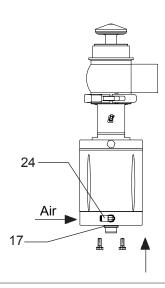
**2.** Fix the guide bushing (17) through 2 screw M6x10 and supply air to fitting (24).
