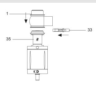
6. Insert the clamp (33) between the lower body (1) and the assembly (35).
