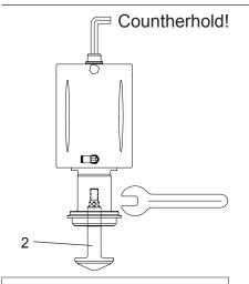
4. Unscrew shutter (2). Counterhold the pivot with an Allen wrench.
