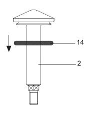
**5a.** Remove the sealing ring (14) from the shutter (2).
