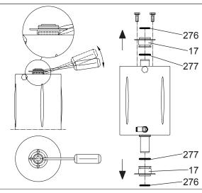
9. Remove screws M6x10 and guide bushing from the cylinder (17) with a suitable tool. Remove seal rings (277 e 276).
