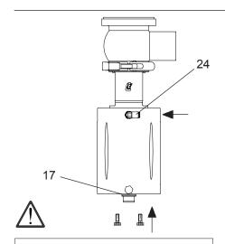
1. Fix the guide bushing (17) through 2 screw M6x10 and supply air to fitting (24).
