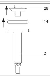
**5b. P.T.F.E. SHUTTER** - Unscrew the shutter nut (28) and remove the sealing ring (14) from the shutter (2).
