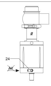
4. Release air pressure to air fitting (24).
