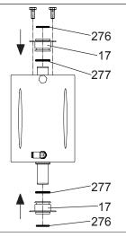
**3.** Insert seal rings (276 e 277) on the guide bushing (17) and assembly them on the cylinder (9) Fix upper guide bushing with two screw M6x10.
