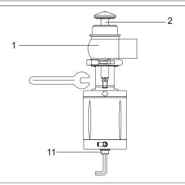
**3.** Unscrew shutter (2). Counterhold the cylinder pivot (11) with an Allen wrench. Remove the shutter (2) from the lower body (1).
