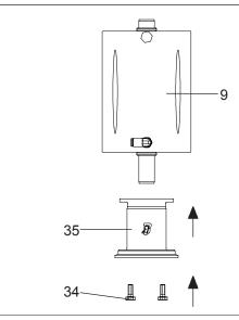
4. Fit assembly (35) to cylinder (9) with screws (34).
