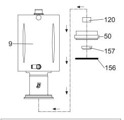
**5.** Insert seal rings (156 e 157)\* and guide bushing (120)\* into the cap (50). Fit the cap on the cylinder (9).
