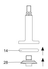
**1.** Pre-heat shutter ring (14\*) to approx. 80°C to make it softer and insert it in shutter slot (2). Insert the ring in a crosswise manner using a plastic cylindrical tool.
