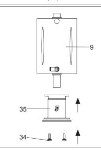
4. Fit assembly (35) to cylinder (9) with screws (34).
