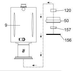
**5.** Insert seal rings (156, 157)\* and guide bushing (120)\* into the cap (50). Fit the cap on the cylinder (9).
