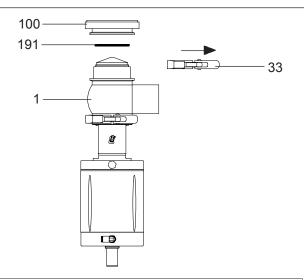
**1.** Remove clamp (33) and split the lower body (1) from the flange (100). Remove the sealing ring (191).
