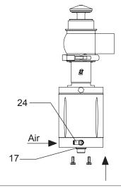
**7.** Screw shutter (2) into cylinder. Counterhold pivot with an allen wrench.
