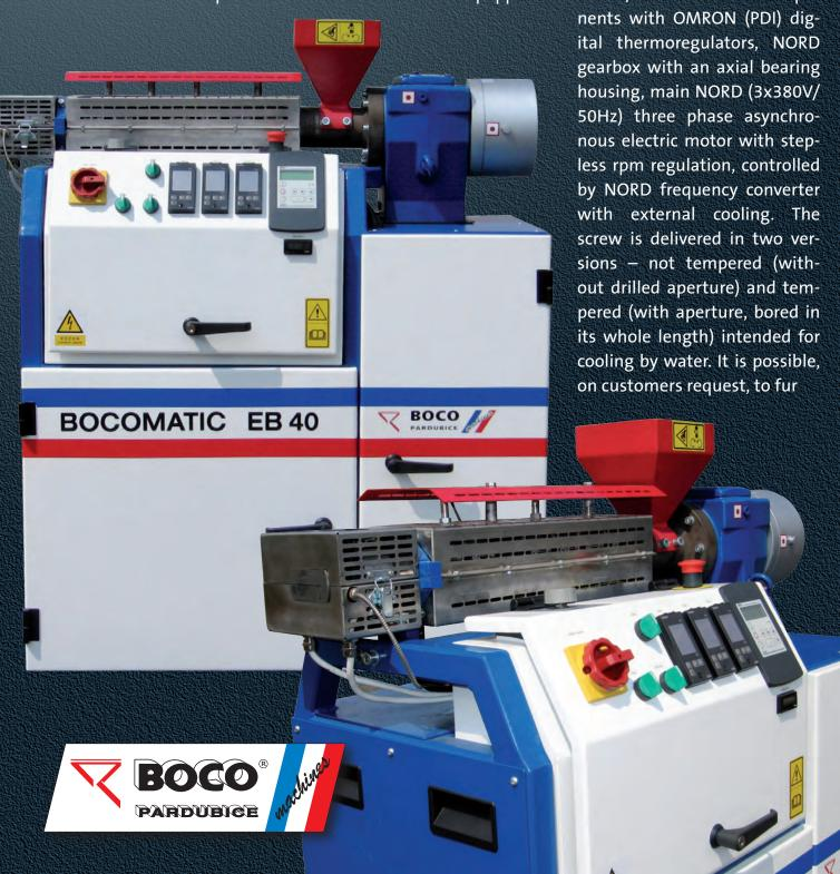
nish the appliance with the MAIER HEIDENHEIM sealing head and with external tempering unit for exact regulation of water temperature. The chamber – working cylinder is equipped with 2 sets of heating zones and cooling zones in the form of sheated barrel intended for cooling by water. The hopper is equipped with a rotary feed roller.
