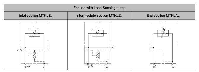
4)Can be used as optional P inlet. Plug unused ports.
