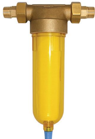
The main components of the protective filter SF are the filter head made of high quality brass, the supporting body with filter stocking and the filter bowl made of high pressure resistant plastic coloured for light stability. Due to its large filtration area, the filter element offers the best possible dirt trapping, economical operation and low maintenance. The filter element meets all hygienical requirements.
