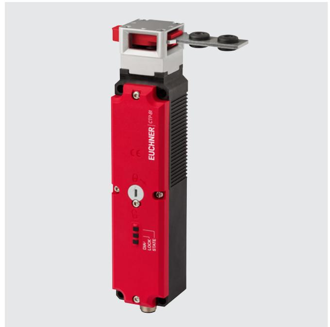
The CTP-BI is based on the proven principle of the safety switch CTP and has an additional bistable locking function. In normal operation the guard locking is controlled via an input signal. When the operating voltage is switched off, the guard locking is maintained in its current position. This means that the safeguarded door remains either locked or unlocked, regardless of locking principle, until power is reapplied.
