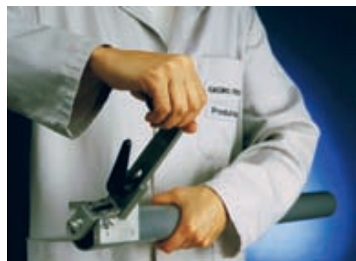
Chamfering the pipe
