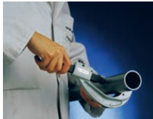
Cutting the pipe to length
