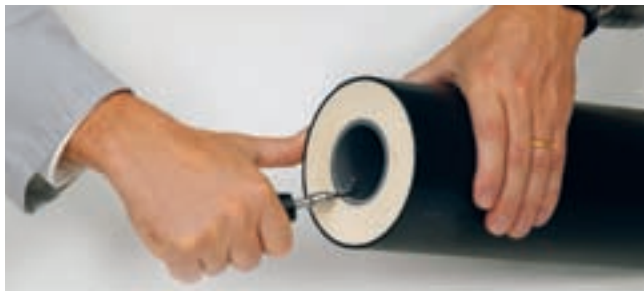
Chamfer to 45° the internal diameter of the ABS pipe.
