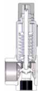
Valve with bellows and gastight cap
