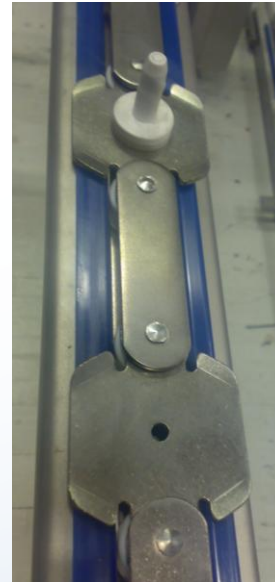
Double side supports for the main chain.
