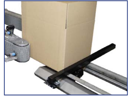
Square Case Transition A pusher bar, parallel to the rear wall of the case, pushes it into the sealing section where spring-loaded side belts automatically adjust for any width variations.
