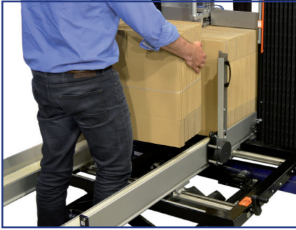
Ergonomic Blank Loading Easy to load magazine. Replenish blanks while machine operates. Simple and fast magazine adjustments.
