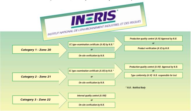
All drive systems offered by LEROY-SOMER are certified by INERIS which endorses their conformity by providing EC TYPE-EXAMINATION CERTIFICATES under the ATEX Directive 94/9/EC.
