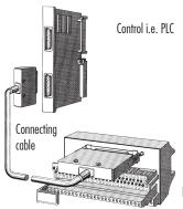
Murrelektronik "passive interface modules" are "plug connectors" — interfaces between the electronics
