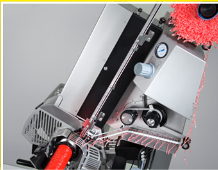
Automatic looper GSE is mounted on the right machine side.
