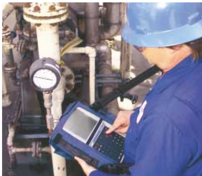
Microlog – portable data collector and analyser
