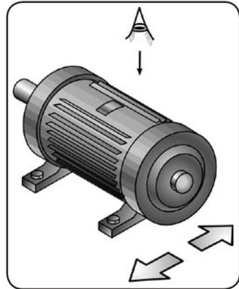
Fig. 24. Horizontal alignment
