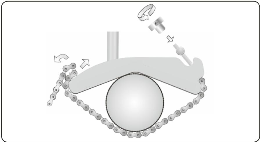
Fig. 8. Attachment of mechanical fixture with chain
