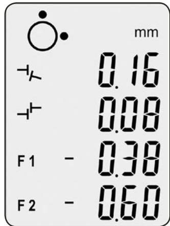
Fig. 21. Display vertical alignment
