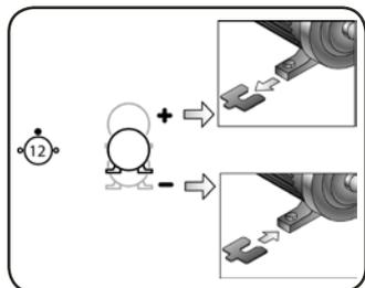
Fig. 22. Vertical alignment
