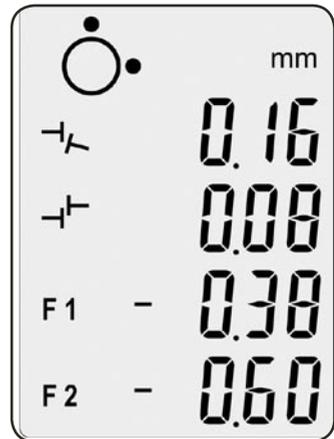
Fig. 19. Measured misalignment
