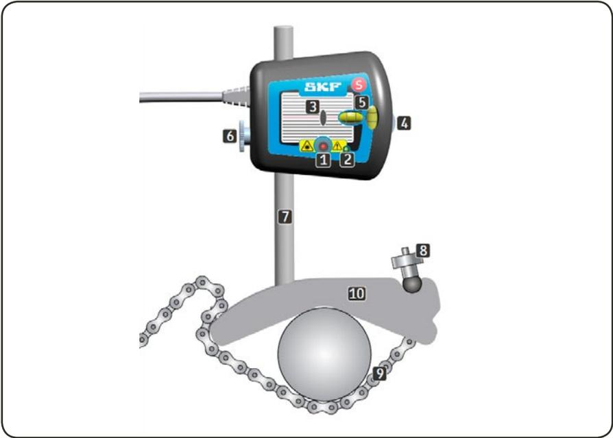
Fig. 7. Mechanical fixture with measuring unit
