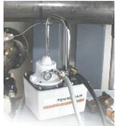
The PA17 used with a flange spreader
