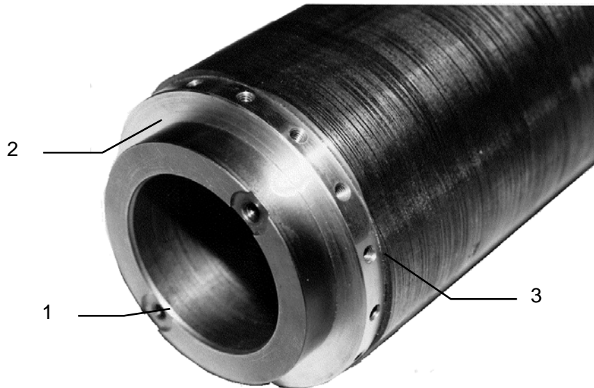
Figure 9: Inlet (1), balancing flange(2) and threaded holes (3)
