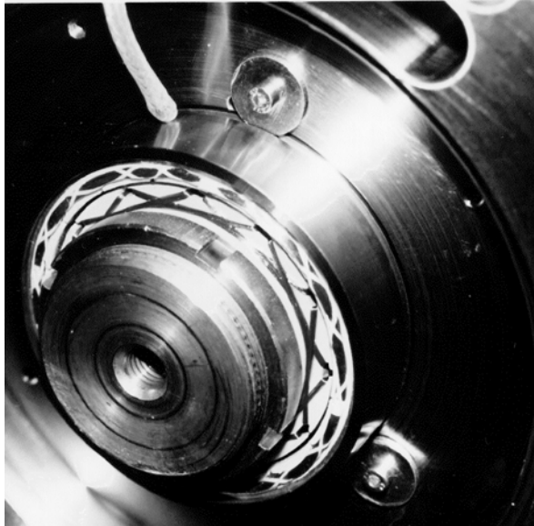
Figure 10: example of resolver mounting
