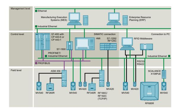
The following communication options are available for connecting SIMATIC MV400/MV500 optical readers to the automation or IT level:
