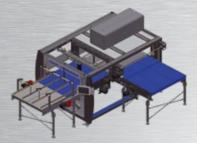
This double-infeed layer composition system comes with two rubberized cadencing belts, two productinsertion belts aimed at forming the row and a one-way translation system that contributes to the formation of the
