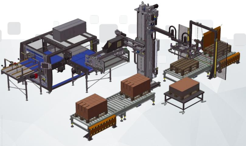
side of the column that remains clear when the packs are inserted into the loading head is exploited by the system for housing the mechanical assembly fitted with SCARA technology, which manages pallet flow and interlayer pad insertion.
