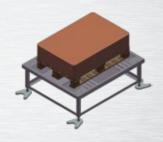
Pad feeding system adjusted according to different interlayer pad sizes.
