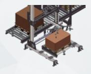
Independent interlayer padinserting device featuring a portal frame. Possibility to directly load the pallet of interlayer pads, provided that it respects alignment limits set for the machine. Side guides to contain interlayer pads are available
