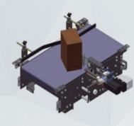
being fed to the palletizer by means of a contrast cylinder. If packs get to the machine with the short side leading, a second optional cylinder is available to ease the rotation process.
