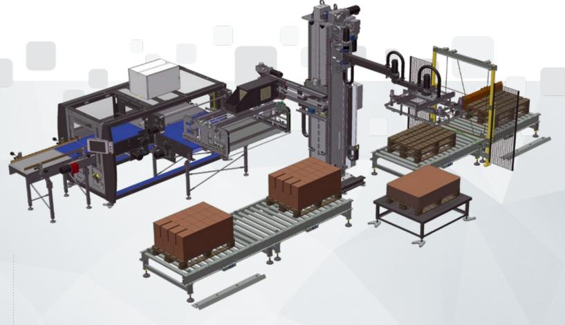
side of the column that remains clear when the packs are inserted into the loading head is exploited by the system for housing the mechanical assembly fitted with SCARA technology, which manages pallet flow and interlayer pad insertion.
