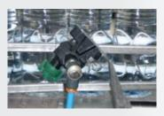
Smiline conveyors are lubricated by an automatic nozzle lubrication system, which minimizes the noise level, the operational costs and the cleaning interventions. It can be supplied "oil free" or
