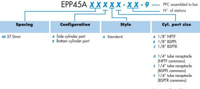
Common (through) ports on manifold are 1/4"
