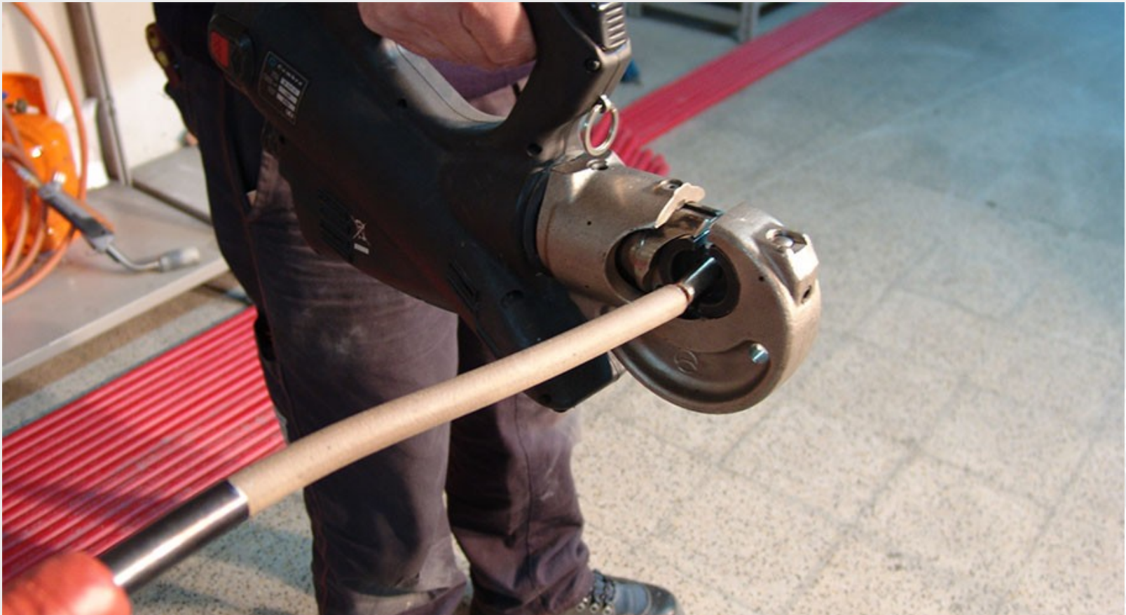
Application of the cable lug
