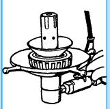
3. Turn the handle of the under 4. Turn on the grease supply valve and fill the bearing with grease. Make sure that the grease is flowing correctly. Turn off the supply valve when finished.
