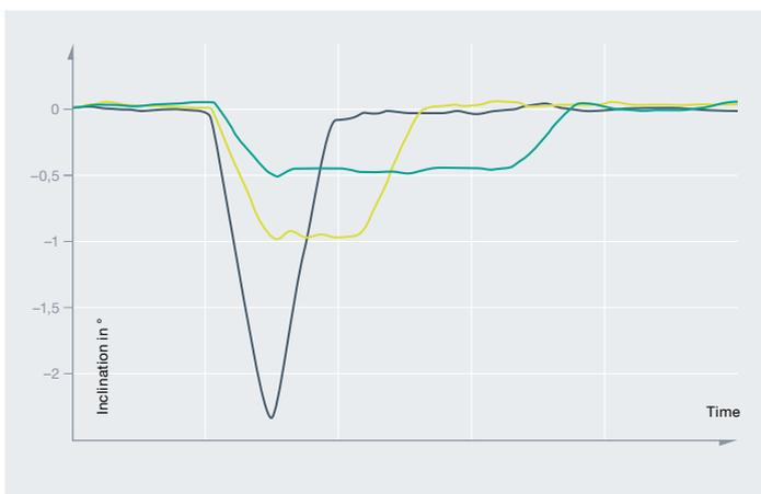
Conventional inclination sensor: measuring error caused by linear acceleration
