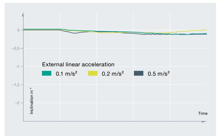
Compensation for external acceleration by F99-Fusion
