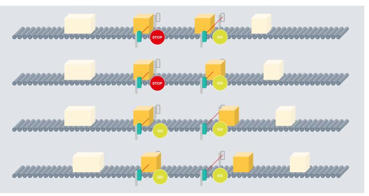
A package may only move downstream if the zone that follows is empty. Zone sensors continuously monitor the flow of packages.
