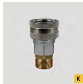
Kupplung : AG. Messing vernickelt + Messing. Max. 250 bar / 150 °C
