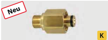
3/8" AG : TR22 IG. K-Lock 6. Messing. Max. 400 bar / 150° C
