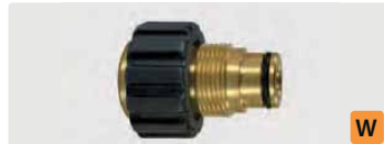
M24 AG : 3/8" IG. Messing *. Max. 400 bar
