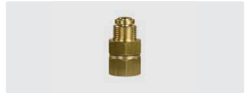
3/8" AG : 1/4" IG. Messing. Max. 220 bar / 90 °C
