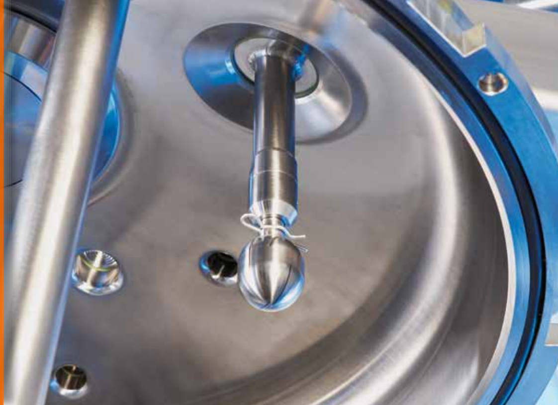
Spray nozzles for a powerful Cleaning In Place
