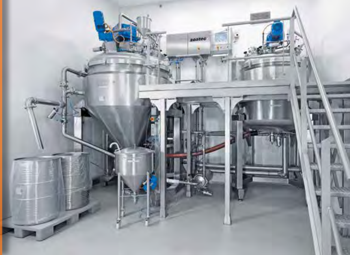
batch vacuum processing plant with separate melt vessel
