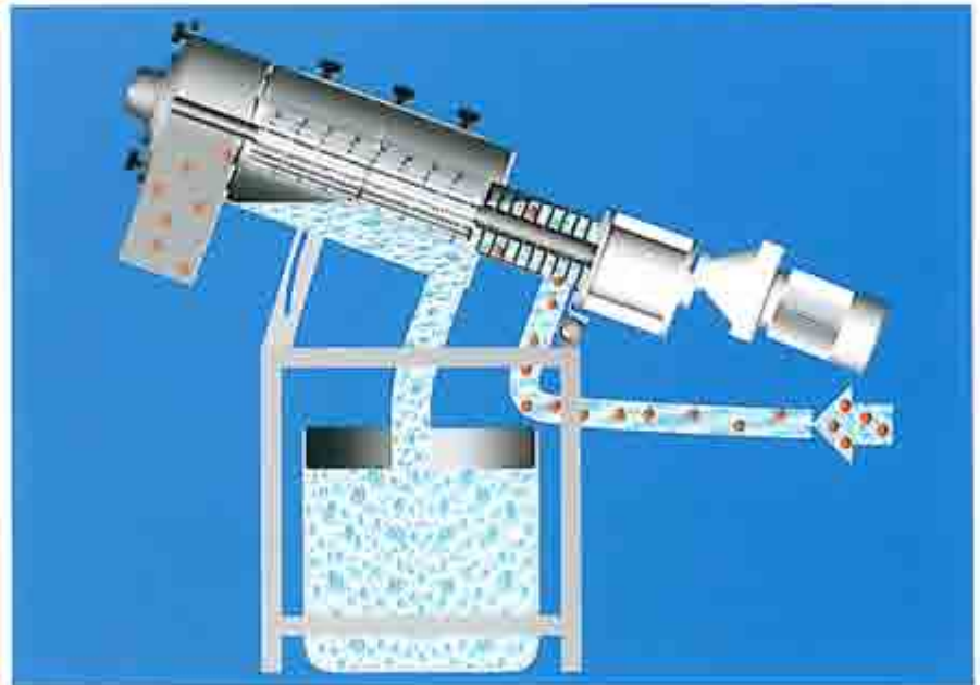
Particles are fed to the solids down spout via the "flow-blades" and removed.
