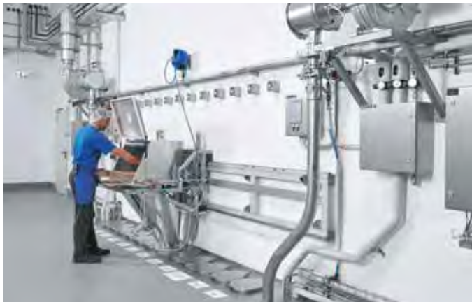
Mobile feeding hopper on the product provision floor for replenishing the surge bin
