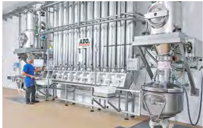
ManDos system with surge bins and two mobile sales in an industrial bakery
