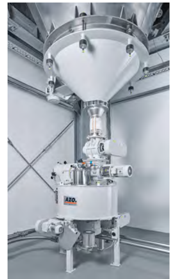
Discharging, screening and distributing flours. Good access underneath the indoor silos
