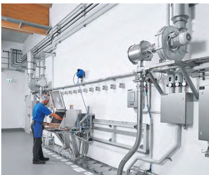
Filling the buffer hoppers via a movable feeding hopper at the feeding level
