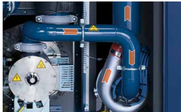
Using warm air from the motor
