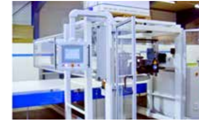
PARKING POSITION: AUTOMATIC PARKING POSITION WITH WATER CLEANING DEVICE
