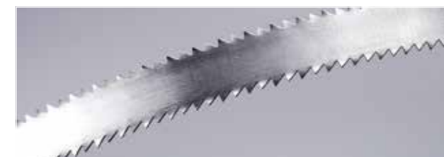
No 21 8 Teeth/inch; 15 x 0,45 mm Double-angle tothing / set
