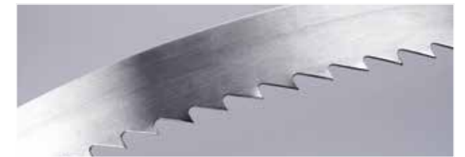
No 25 3 Teeth/inch; 20 x 0,50 mm Angle tothing / set with broaching tooth
