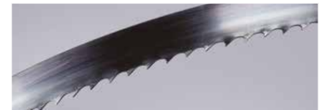
No 27 4 Teeth/inch; 20 x 0,50 mm Angle tothing / set with broaching tooth
