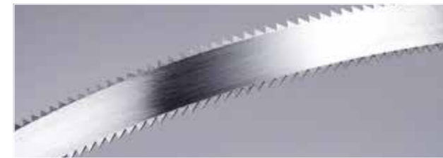
No 37 | 10 Teeth/inch; 15 x 0,45 mm | Double angle tooting
