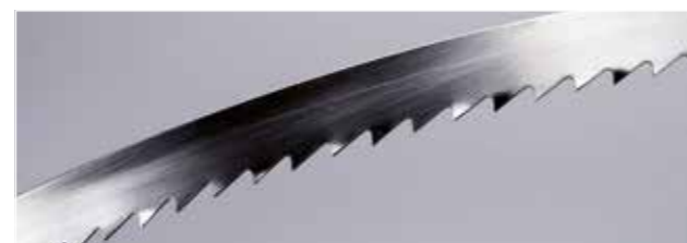
No 23 4 Teeth/inch; 13 x 0,50 mm Angle tothing / set with broaching tooth
