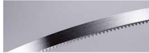
No 30 | 10 Teeth/inch; 10 x 0,45 mm | Pointed tooting
