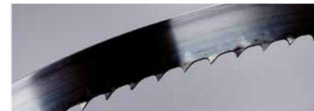
No 26 3 Teeth/inch; 20 x 0,80 mm Angle tothing / set with broaching tooth
