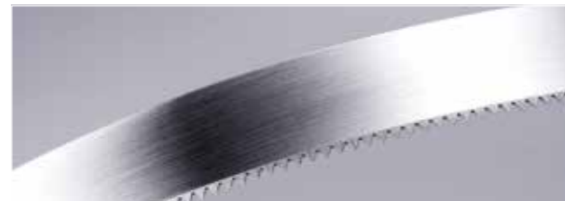
No 34 | 10 Teeth/inch; 20 x 0,45 mm | Pointed tooting
