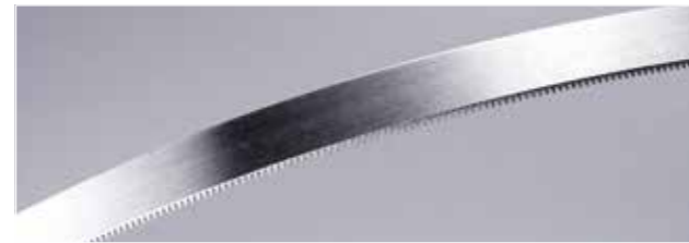
No 14 | 25 Teeth/inch; 10 x 0,45 mm | Pointed tooting
