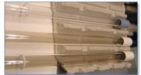
UV output measured from the brand new Competitor lamps was 5.50mW/cm<sup>2</sup> and the UV output measured from the aged Competitor lamps was 3.28 mW/cm<sup>2</sup> at about 4,000 hours. This corresponds to a UV output decrease of >40% after only 4,000 hours, which is less than 6 months of lamp operation.
