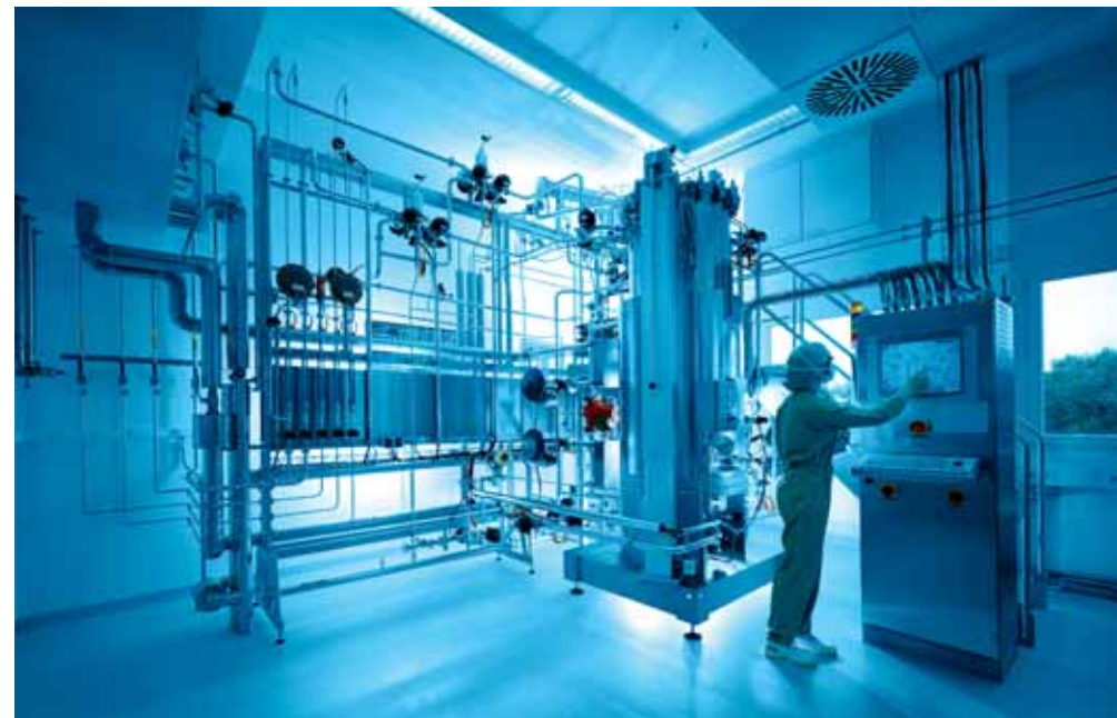
Main production bioreactor, capacity 500 liters.
