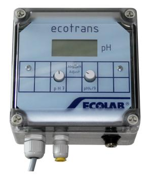
The ECOTRANS pH measurement transmitter records measurements in a range from pH 2 to pH 12 and converts these into a 4-20 mA standard signal (pH 2 = 4 mA, pH 12 = 20 mA).
