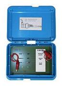
**Calibration box** for conductivity measurement (conductive) with simulation resistances for the measurement ranges 0 - 2, 0 - 20, 0 - 200 µS/cm
