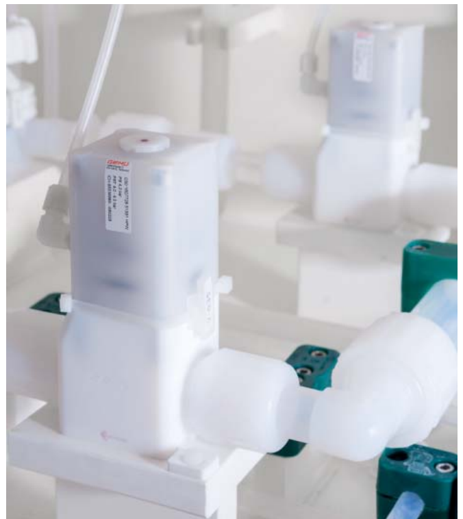
Plant in the semiconductor industry with GEMÜ iComLine® valves
