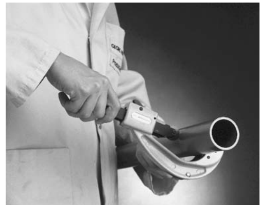
Cutting the pipe to length
