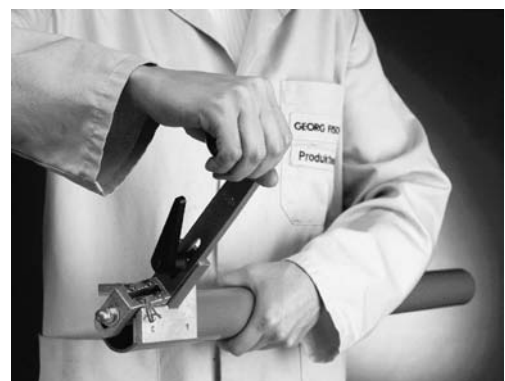
Chamfering the pipe
