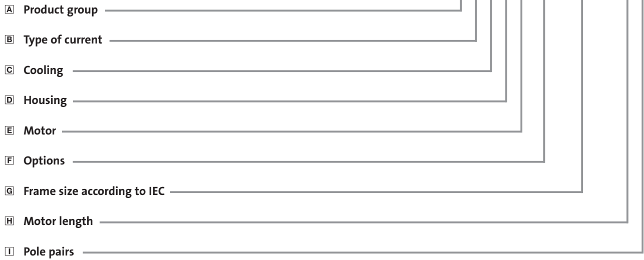
Key to 931M servo drives type code; consisting of 931M servo inverter and SDS motor
