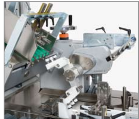
Rotary carton erection with "standing still" positions for picking, pre-breaking and opening of the cartons.
