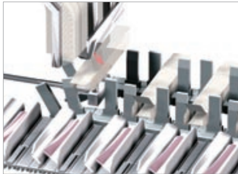
Carton erection by oscillating arm.
