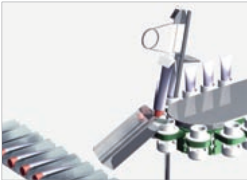
Cap first tube discharge (intermittent working machine).
